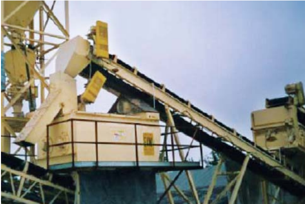
Figure 29. Pugmill used to mix hydrated lime with the wet aggregate in South Carolina (USA) (from [145]).
